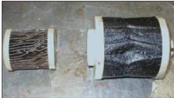
Improperly Maintained Fuel Filters
